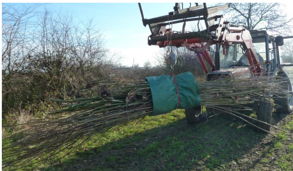
Figure 4. Weighing willow sample with tractor-mounted spring balance
